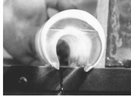
Figure 2. Photo of cross-section of an ice shell after melting through.
